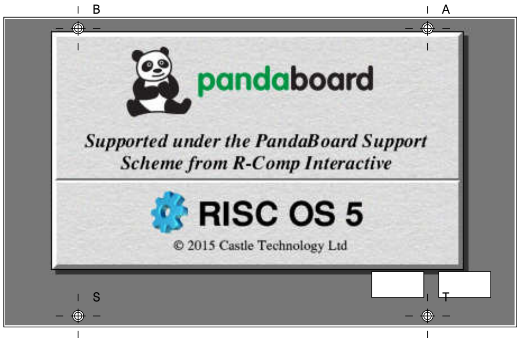
FRONT 84x138x2 Holes ABST 6BA csk Cutout for USB hub
