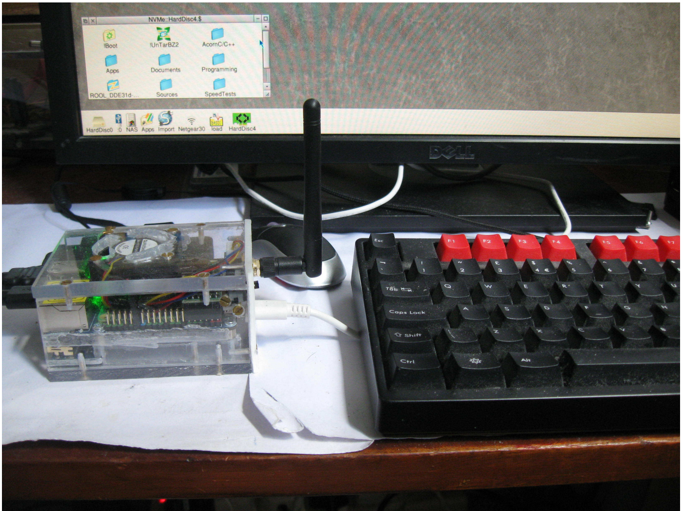
Here we have a Waveshare IO board with 4GB CM4 with eMMC, 4 USB sockets, 2 HDMI sockets, Ethernet socket, a Sabrent 512GB NVMe drive, connected securely using WiFi.
